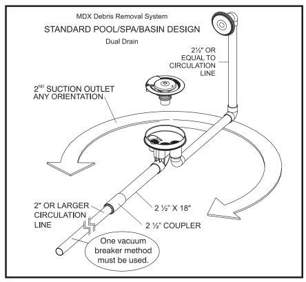
Spa Systems includes the 18 inches of 2½" pipe plus coupler with the MDX Debris Removal System. To order separately, please see page 8 for the part number.
